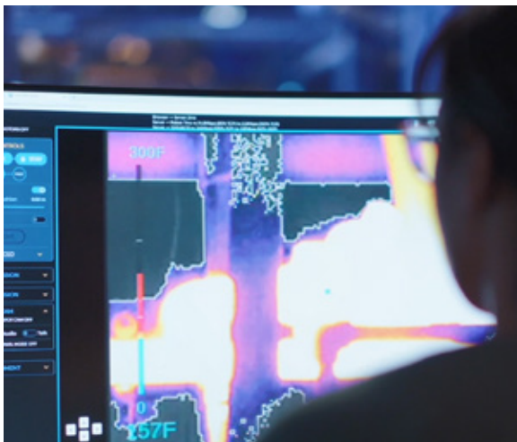
Thermal imaging payloads mounted to Boston Dynamics' legged robot platforms can reveal high-low temperature conditions indicative of early equipment failure or inadequate heating for material process applications, among many other industrial use cases.
